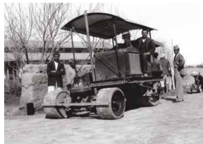
A Barford & Perkins D4 type motor roller is summonsed to hopefully rescue the unfortunate steam roller.
