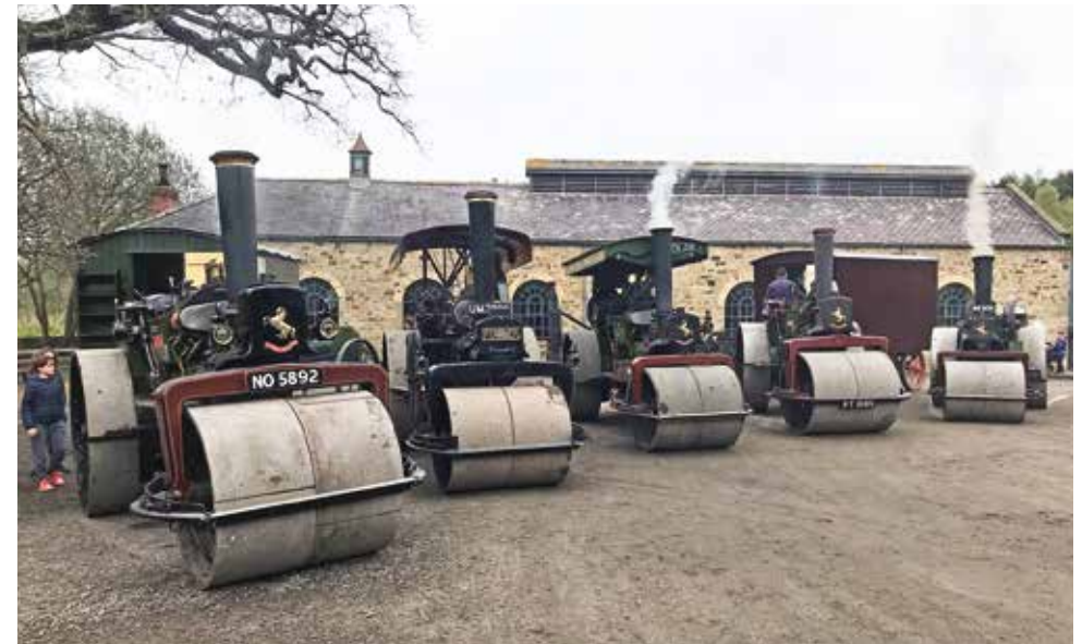
From left to right: James West's 10 ton Aveling & Porter F Type compound No.10346 of 1922 Buster; Mark & Chris Bainbridge's Fowler No.16615 of 1925 Astonisher; Tony and Andrew Borthwick's Aveling & Porter 8 ton D Type compound No.11145 of 1925 Ayesha; Andrew Cook's 10 ton E Type No.10707 of 1923 Pegasus; Dave Bickerdike's Aveling & Porter R6 No.5499 of 1904.
